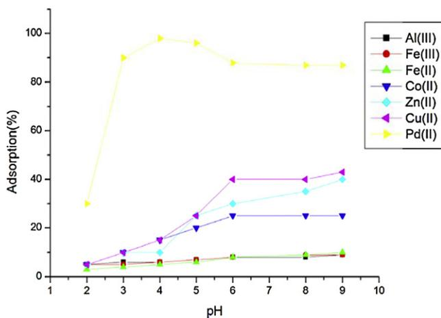
Fig. 3. Effect of pH on adsorption of Al(III), Fe(II), Fe(III), Co(II), Zn(II), Cu(II) and Pd(II) onto DKTS-APSG resin. 50 mg resin, 10 ml test solution.
