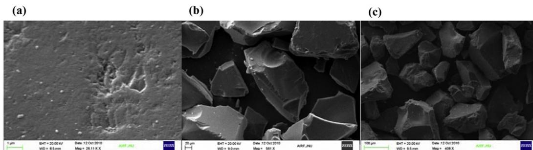
**Fig. 2.** SEM images of fresh DKTS–APSG chelating resin, (a) at high magnification (26.11K $\times$ ) (b) at low magnification (561 $\times$ ), and (c) the resin reused for 10 cycles (Magnification 408 $\times$ ).
