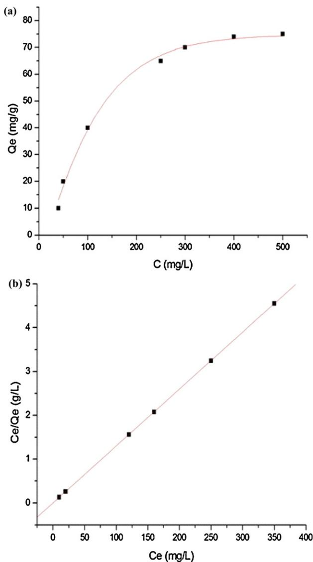
Fig. 4. (a) Adsorption isotherm of Pd(II) ions onto DKTS-APSG and (b) the linear form of the Langmuir adsorption isotherm. 100 mg resin, 50 ml test solution, pH 4.
